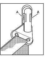
To move it up or down, squeeze the release buttons (A) together and move the height adjuster to the desired position.
